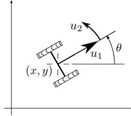
Figure 3.4: The unicycle, as studied here, has three generalized coordinates  $(x, y, \theta)$ , corresponding to location and heading, and two control inputs  $u_1$  and  $u_2$  that correspond to linear speed and rotational speed, respectively.
