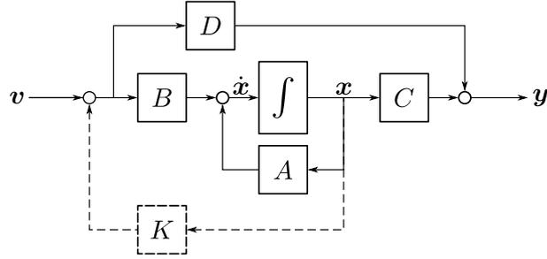
Figure 4.7: Feedback control loop (dashed lines) attached to the linear system.
