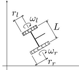
Figure 3.5: The unicycle with wheel rotational speed control inputs.
