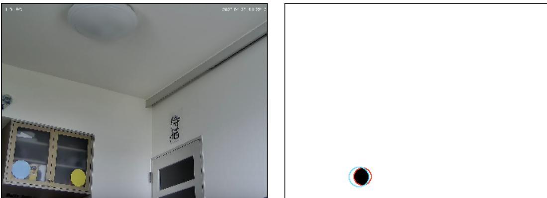
Figure 7.7: Image and processing output of the first, unsuccessful approach to detect the position of the beacons based on the Hough transform.
