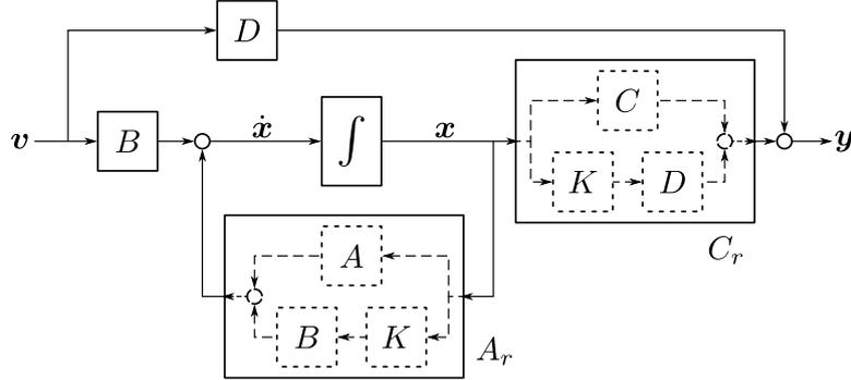
Figure 4.8: Graphical representation of the feedback-controlled linear system converted into the canonical representation.
