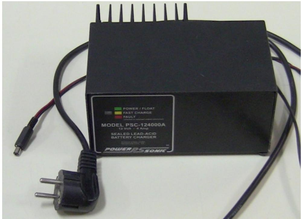
Figure 4.16: Robot base charger.
