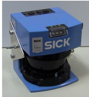
Figure 4.4: Laser sensor.
