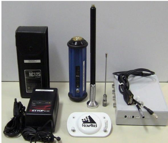
Figure 4.9: Differential GPS set. Rover station parts.
