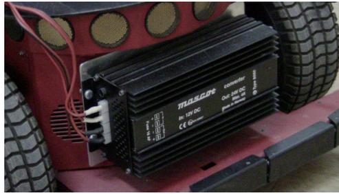
Figure 4.8: 12V to 24V converter.
