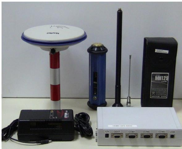
Figure 4.10: Differential GPS set. Base station parts.
