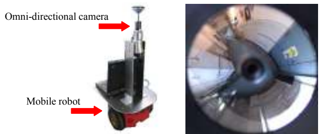
Fig.1 Mobile Robot and Omni-directional Image
