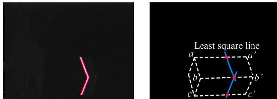
(a) Laser image. (b) Extracted lines.
