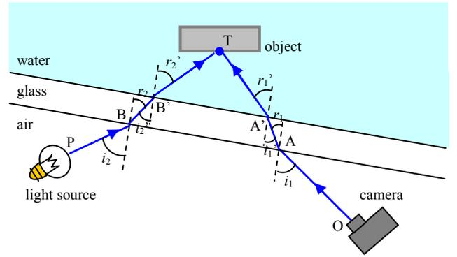
Fig. 5 3-D measurement model
