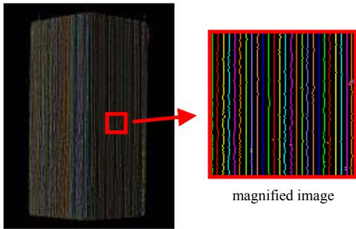
Fig. 10 Encoded image (white pentagonal prism)
