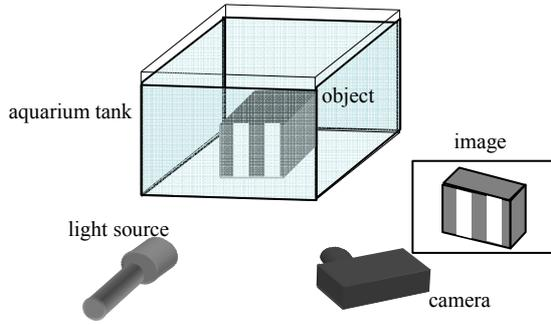
Fig. 2 Measurement of an underwater object by space encoding method
