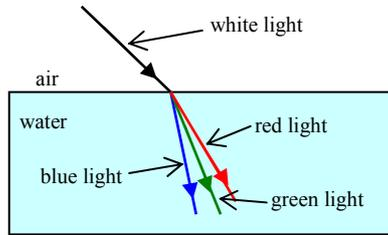
Fig. 3 Refraction of white light
