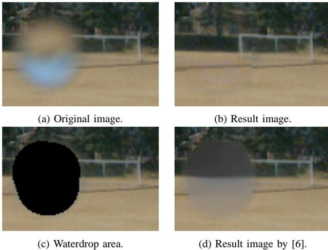
Fig. 10. Example of waterdrop removal.
