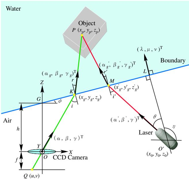
Fig. 6. Principle of 3-D measurement.
