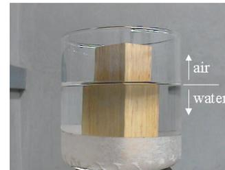
Fig. 2. Example of image distortion (size and shape change).
