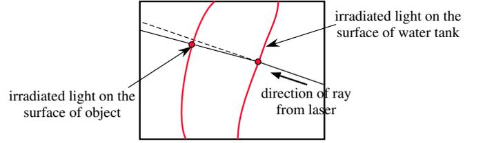
Fig. 7. Extraction of laser point.
