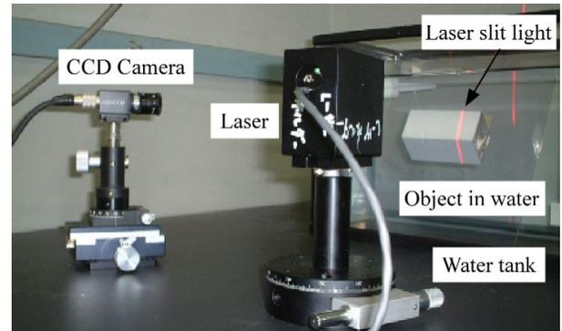
Fig. 4. Overview of 3-D measurement by using the light stripe projection method.
