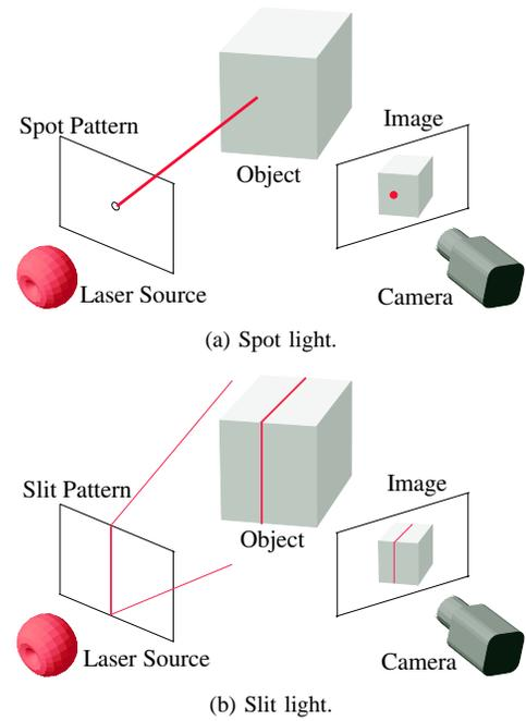
Fig. 3. 3-D measurement with laser range finders.
