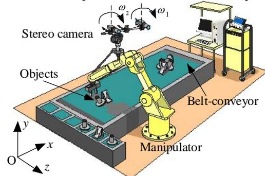
Fig.1 The manipulator handles moving objects.
