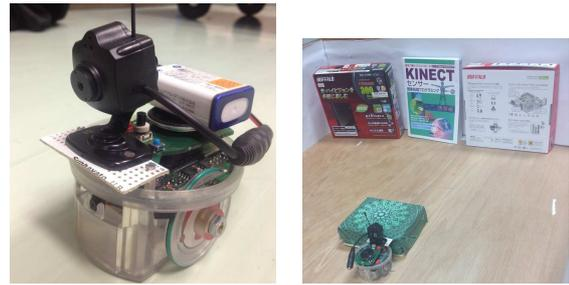
(a) Mobile robot with CCD camera. (b) Robot, object and environment
